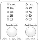
Press the Spin button repeatedly to change the spin speed, if you want your laundry to be spun at a speed different from the one proposed by the appliance.
